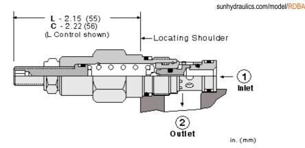
Direct-acting relief cartridges are normally closed, pressure-limiting valves used to protect hydraulic components from pressure transients. When the pressure at the inlet (port 1) reaches the valve setting, the valve starts to open to tank (port 2), throttling flow to limit the pressure rise. These valves are smooth and quiet, essentially zero leak, dirt tolerant, immune to silting and are very fast.
