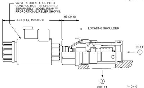
This valve is a normally closed modulating element that incorporates an integral pilot control cavity. It is a balanced piston design. The pilot control cavity will accept any T-8A pressure control cartridge. When the pressure at the inlet (port 1) reaches the pilot control cartridge's setting, the modulating element starts to open to tank (port 2), throttling flow to regulate the pressure. The pilot cartridge's setting determines the difference in pressure between port 1 and port 2.
