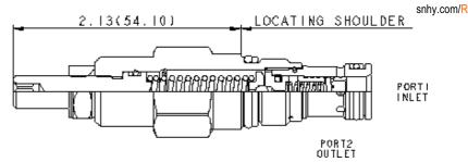
Pilot-operated, balanced-piston relief cartridges are normally closed pressure regulating valves. When the pressure at the inlet (port 1) reaches the valve setting, the valve starts to open to tank (port 2), throttling flow to regulate the pressure. These valves are accurate, have low pressure rise vs. flow, they are smooth and quiet, and are moderately fast.
