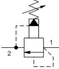
Pilot-operated, balanced-piston relief cartridges are normally closed pressure regulating valves. When the pressure at the inlet (port 1) reaches the valve setting, the valve starts to open to tank (port 2), throttling flow to regulate the pressure. These valves are accurate, have low pressure rise vs. flow, they are smooth and quiet, and are moderately fast.
