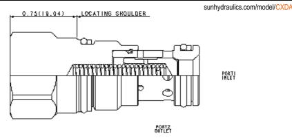
Free-flow, nose-to-side check valves are on/off circuit components that allow free flow from the inlet (port 1) to the outlet (port 2) and block flow in the opposite direction.
