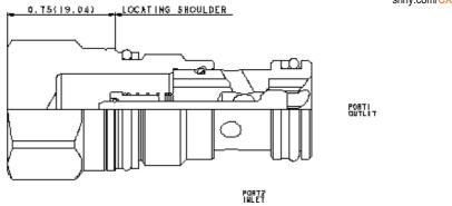
Free-flow, side-to-nose check valves are on/off circuit components that allow free flow from the inlet (port 2) to the outlet (port 1) and block flow in the opposite direction.
