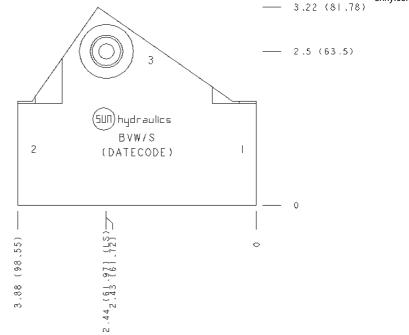
Pilot-operated, balanced-piston relief cartridges are normally closed pressure regulating valves. When the pressure at the inlet (port 1) reaches the valve setting, the valve starts to open to tank (port 2), throttling flow to regulate the pressure. These valves are accurate, have low pressure rise vs. flow, they are smooth and quiet, and are moderately fast.
