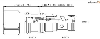
This valve is a pilot to open check valve. It has a non-sealed pilot, a steel seat, and is non-vented. It allows free flow from the valve (port 2) to the load (port 1) and blocks flow in the opposite direction. Pressure at the pilot (port 3) will open the valve from port 1 to port 2. Pilot pressure needed at port 3 to open the valve is directly proportional to the load pressure at port 1. Pressure at port 2 directly opposes pilot pressure.
