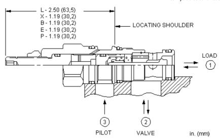
This valve is a pilot to open check valve. It has a non-sealed pilot, a steel seat, and is non-vented. It allows free flow from the valve (port 2) to the load (port 1) and blocks flow in the opposite direction. Pressure at the pilot (port 3) will open the valve from port 1 to port 2. Pilot pressure needed at port 3 to open the valve is directly proportional to the load pressure at port 1. Pressure at port 2 directly opposes pilot pressure.
